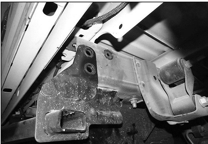
(Fig 7) End of frame once factory bumper is removed. Passenger side with receiver hitch pictured
