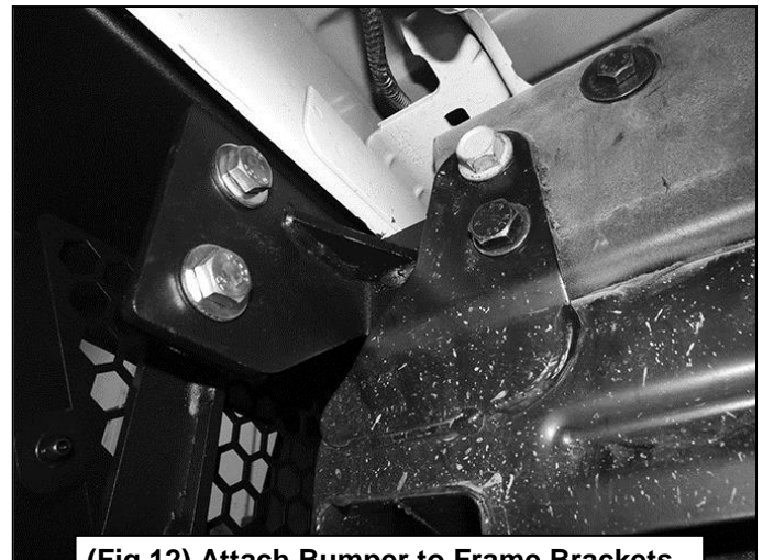
(Fig 12) Attach Bumper to Frame Brackets
