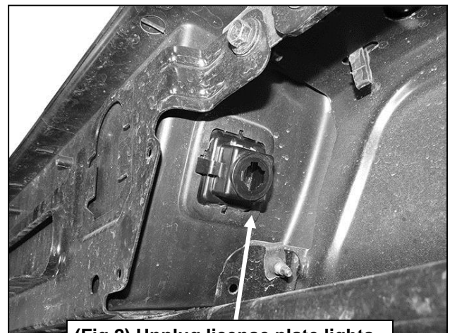
(Fig 2) Unplug license plate lights
