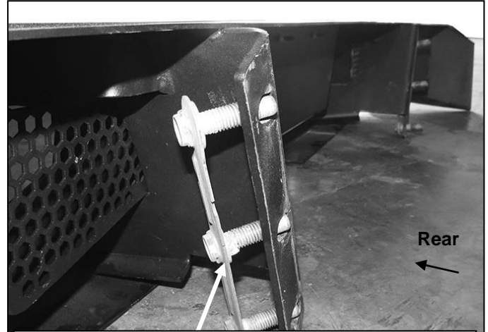
(Fig 4) On models without receiver hitch, reuse triple bolt plate to attach bumper to ends of frame
