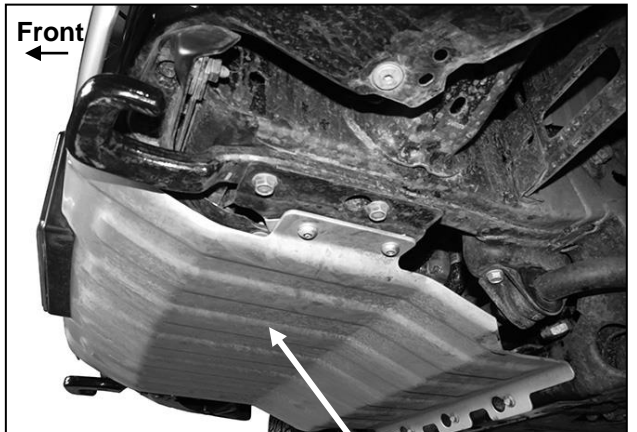
(Fig 4) Remove skid plate if equipped
