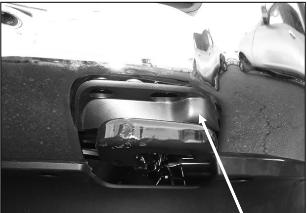
(Fig 3) Remove plastic panel above tow hook
