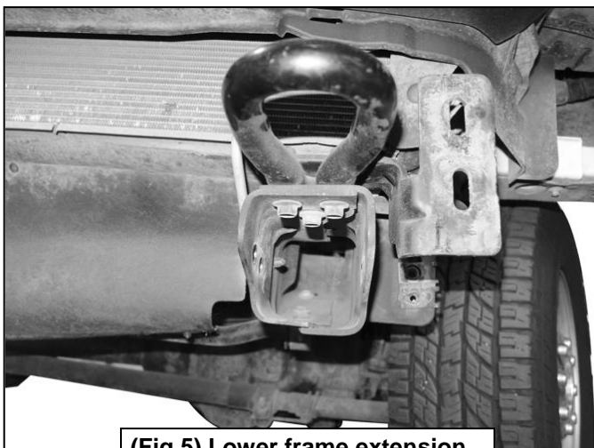
(Fig 5) Lower frame extension removed on driver side
