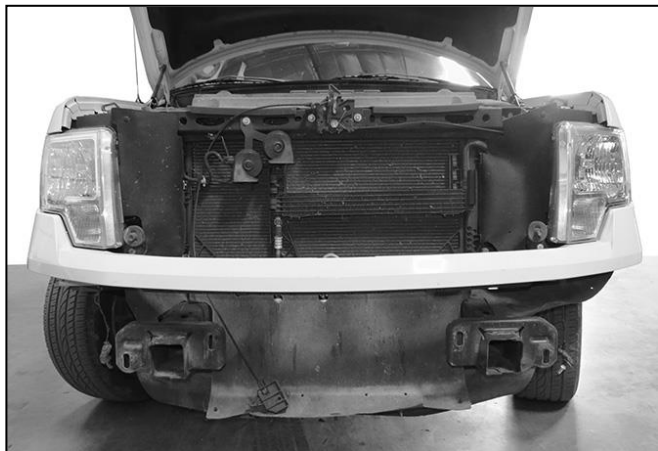
(Fig 6) Remove bumper assembly. Also remove tow hooks and double nut plates if equipped
