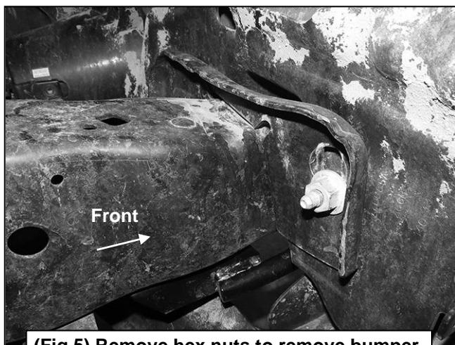
(Fig 5) Remove hex nuts to remove bumper
