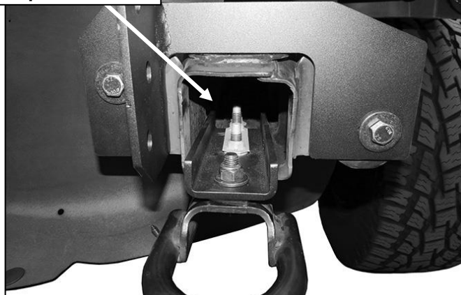
(Fig 9) Tow hook attached to Relocation Bracket
