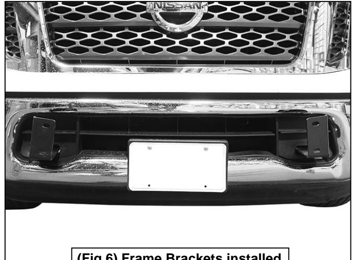
(Fig 6) Frame Brackets installed
