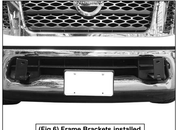
(Fig 6) Frame Brackets installed
