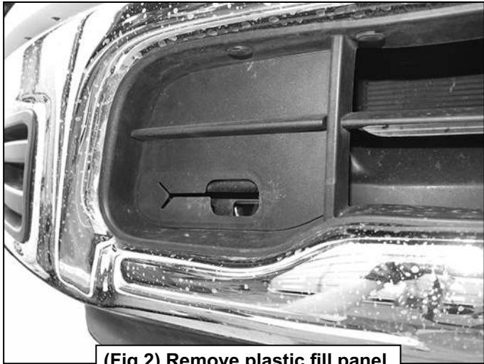
(Fig 2) Remove plastic fill panel
