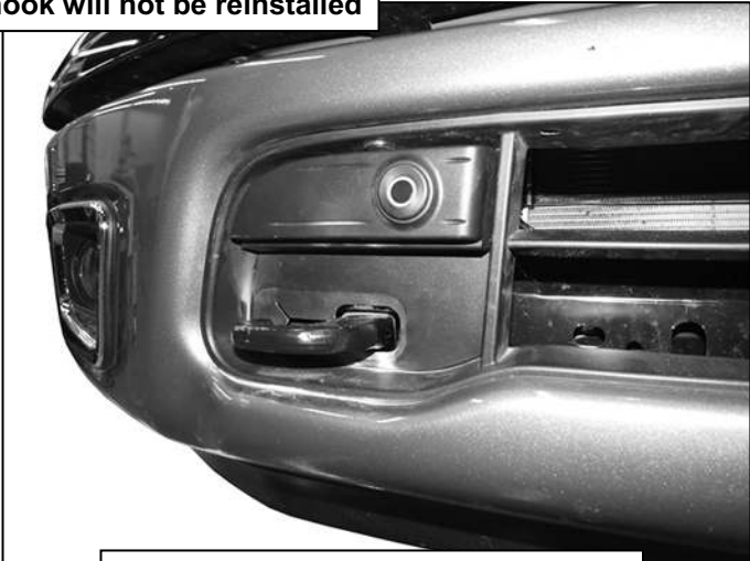
(Fig 3) Remove tow hook if equipped
