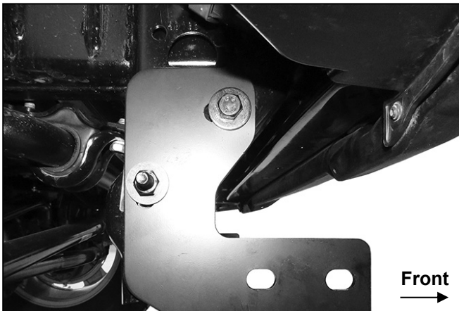
(Fig 5) Passenger/right Frame Bracket installed
