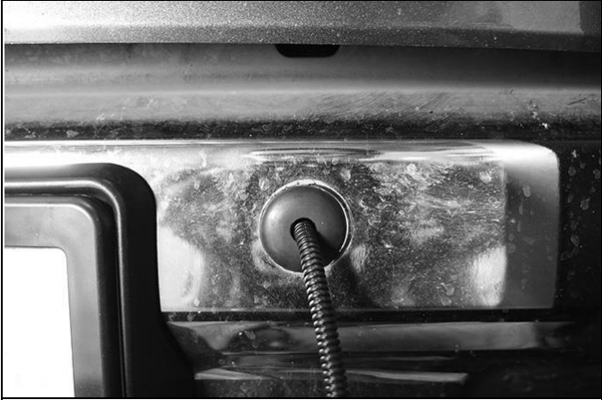
(Fig 21) Models with sensors, slide Grommet over small end of Harness Extension. Push Grommet into hole in bumper and attach to wiring harness
