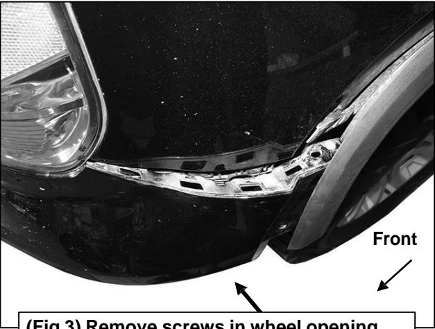
(Fig 3) Remove screws in wheel opening. Carefully pull to release fender flare and to remove fascia if equipped (arrow)
