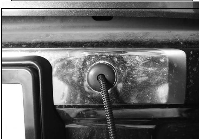
(Fig 21) Models with sensors, slide Grommet over small end of Harness Extension. Push Grommet into hole in bumper and attach to wiring harness
