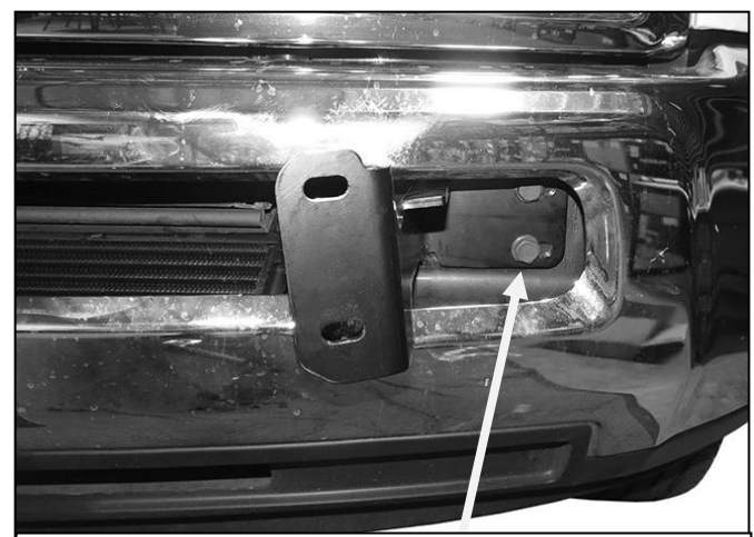
(Fig 4) Driver/Left Side Mounting Bracket Installed
