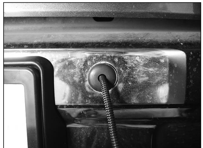
(Fig 14) Models with sensors, slide Grommet over small end of Harness Extension. Push Grommet into hole in bumper and attach to wiring harness
