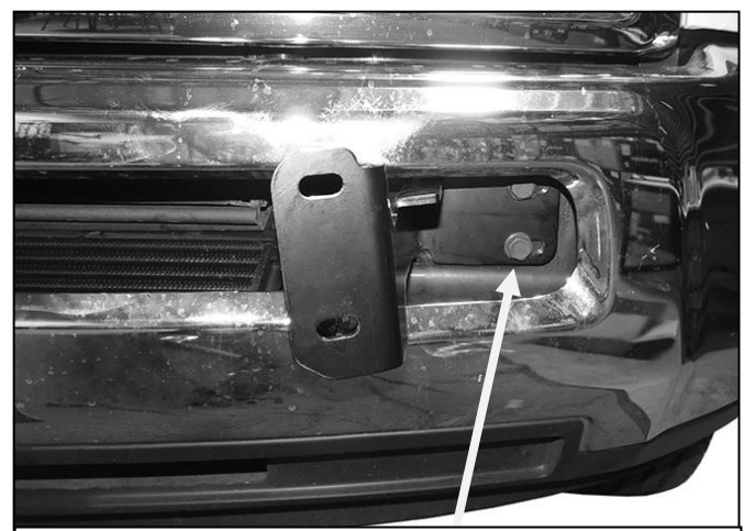
(Fig 4) Driver/Left Side Mounting Bracket Installed
