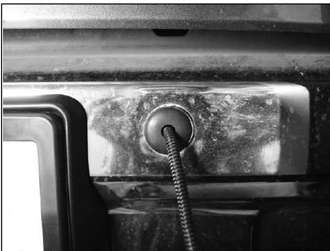
(Fig 21) Models with sensors, slide Grommet over small end of Harness Extension. Push Grommet into hole in bumper and attach to wiring harness
