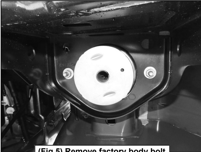
(Fig 5) Remove factory body bolt
