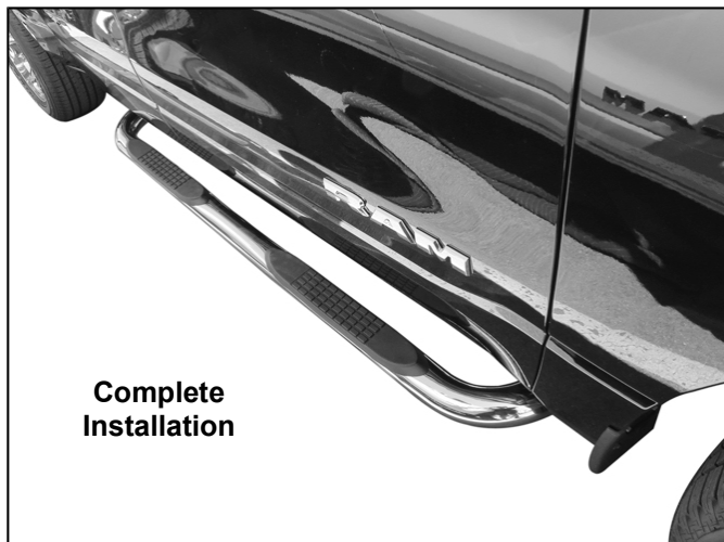
(Fig 12) Driver/left Front Brackets and Sidebar installed
