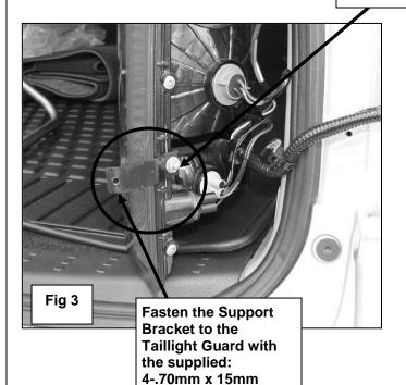
Phillips Head Screw 4mm Flat Washer 4mm Lock Washer
