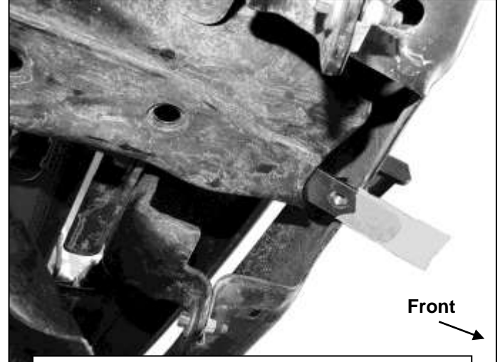
(Fig 8) Models w/o tow hooks, insert Nut Plate into end of frame. (Note: pictured without plastic lower air dam for instructions only)
