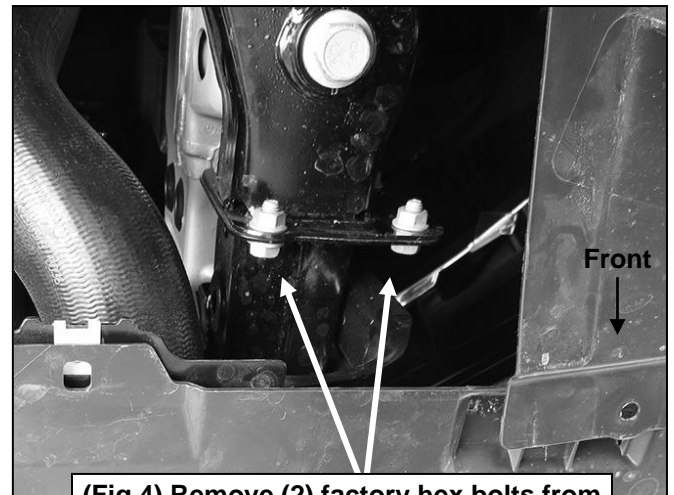
(Fig 4) Remove (2) factory hex bolts from bottom of frame rail/bumper bracket
