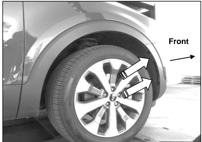
(Fig 2) Remove the factory plastic grille, bolts and clips. Place them on a clean, stable work area.
