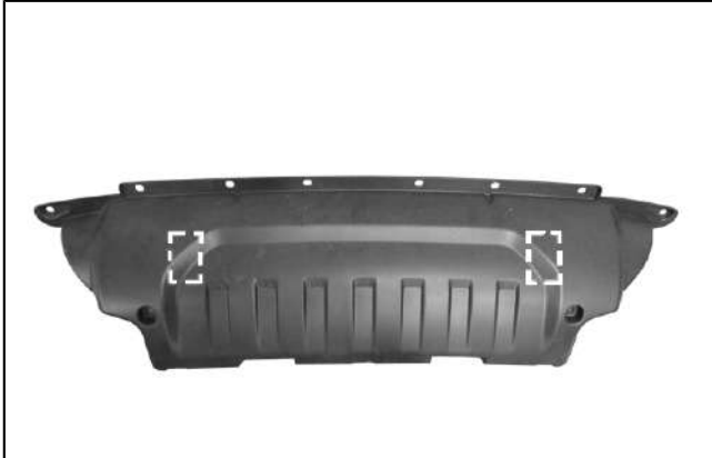
(Fig 15) Trim the approximate area to clear the Mounting Brackets through the splash guard
