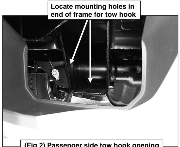
Locate mounting holes in end of frame for tow hook
