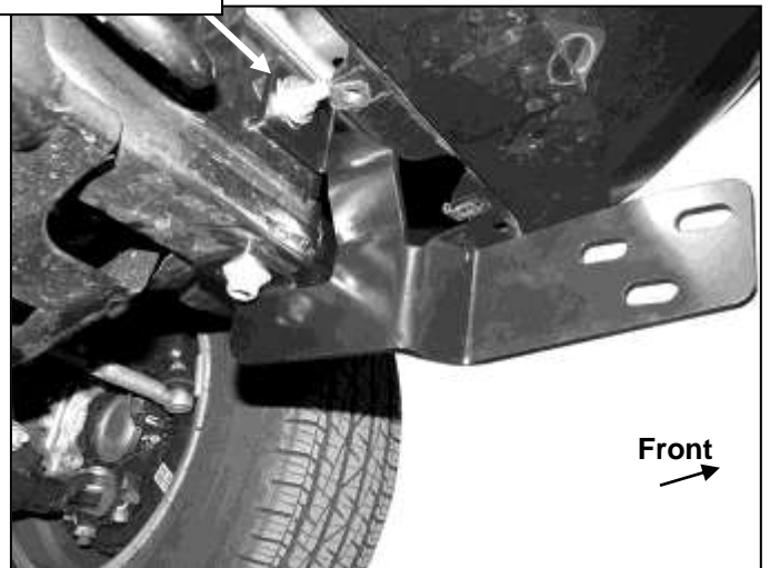
(Fig 6) Driver side Frame Bracket installed
