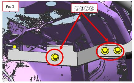
Step4: Check if all hard ware are installed and fastened. Step 5: Complete the installation.
