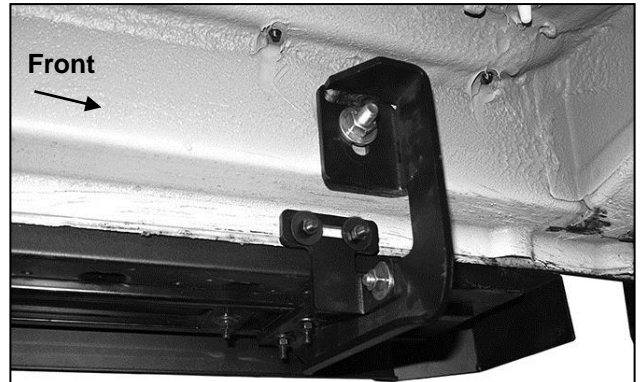
(Fig 18) Driver/left Front Brackets installed
