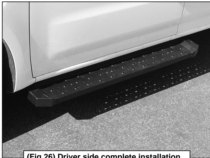
(Fig 26) Driver side complete installation
