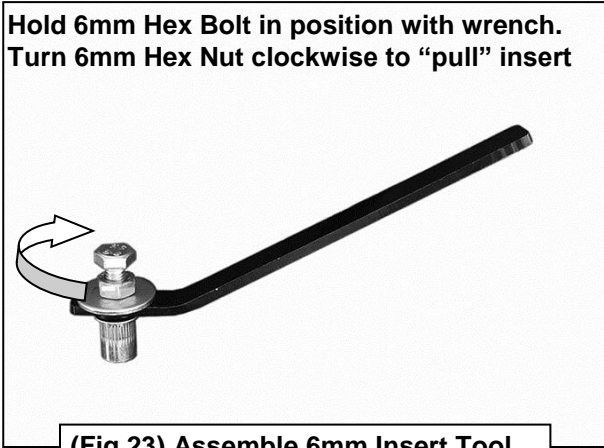
(Fig 23) Assemble 6mm Insert Tool
