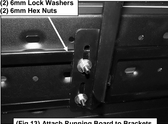
(Fig 13) Attach Running Board to Brackets
