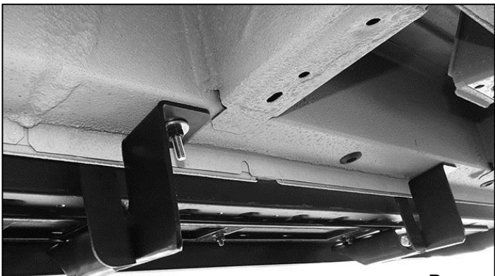
(Fig 21) Passenger side Bracket layout w-Support Brackets
