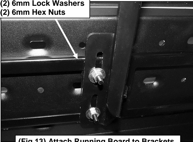
(Fig 13) Attach Running Board to Brackets
