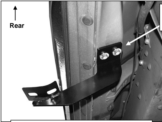
(Fig 5) Driver/Left Rear Bracket installed
