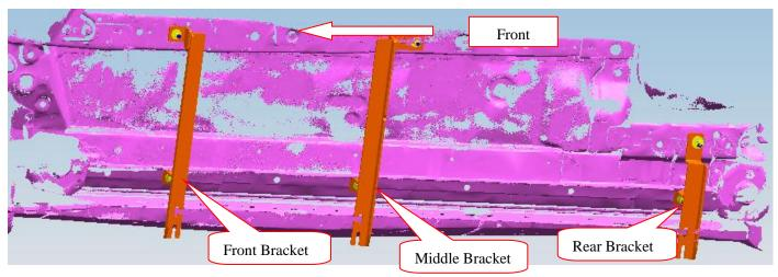
Step 3: Install the running board on the brackets and then adjust them to the proper positions.
