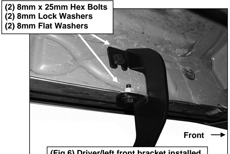
(Fig 6) Driver/left front bracket installed
