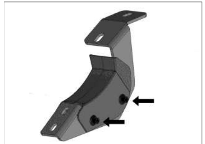
(Fig 4) Push center pin in to expand Clip in Bracket
