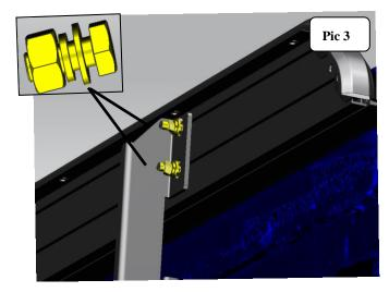
Step 4: Refer to Pic 3 to install V1 Running Board with running board hard ware. Step 5: Check if all hard ware are installed and then fasten all to complete the installation.
