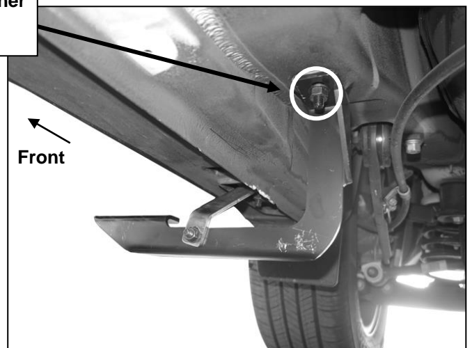
(Fig 10) Passenger side rear bracket installed
