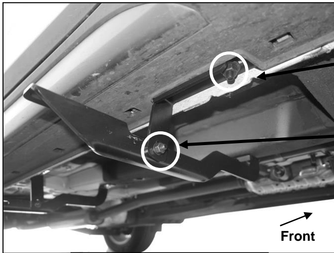
(Fig 7) Passenger side Front Support Bracket installed
