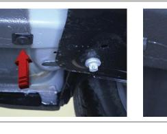
Place an L-shaped hanger bracket onto the vehicle and secure with an M8 flat washer, M8 lock washer and M8 hex nut.
