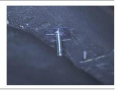
Locate and remove the hole plug in the rocker panel. Insert an M8 T-bolt plate into the opening. Slide a plastic bolt retainer over the thread of the bolt to hold the bolt in place.
