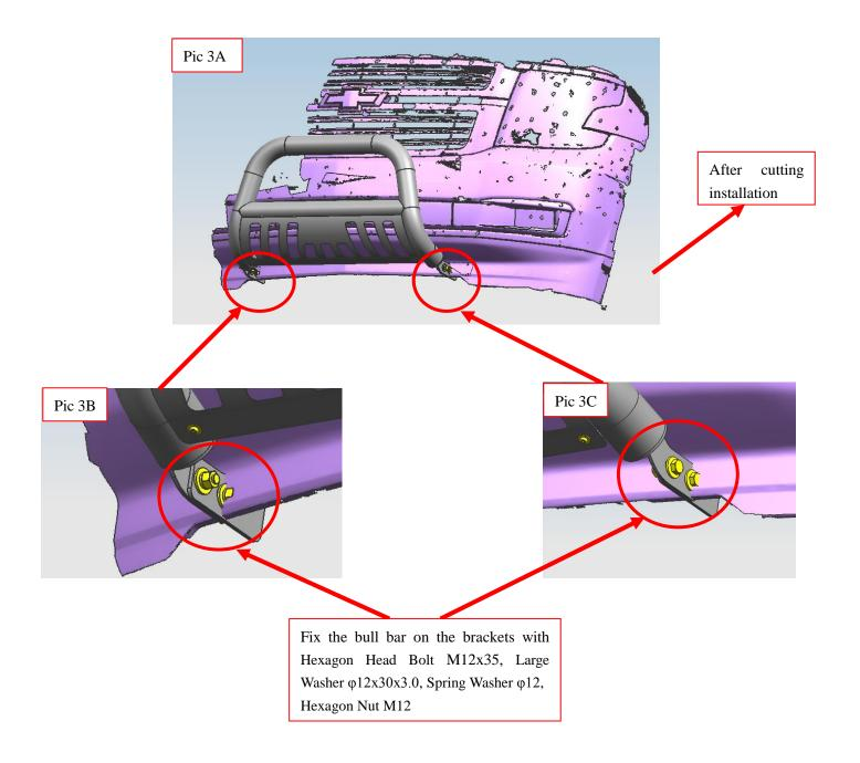
Step 3: Install the bull bar on the brackets and then adjust the brackets to the proper position.
