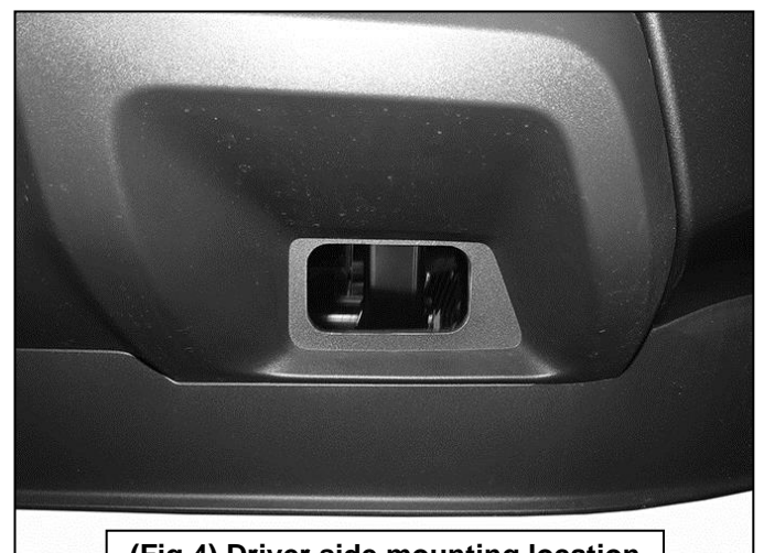
(Fig 4) Driver side mounting location
