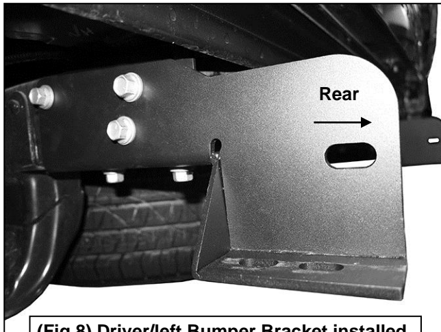
(Fig 8) Driver/left Bumper Bracket installed
