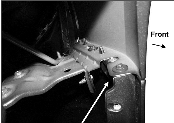
(Fig 6) Remove hardware attaching bumper cover to fender. Remove bumper cover
