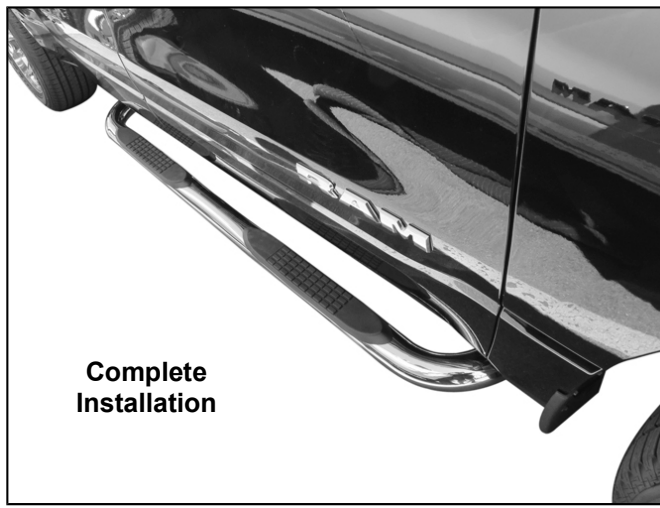
(Fig 12) Driver/left Front Brackets and Sidebar installed
