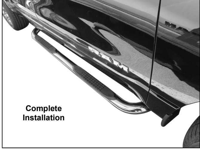
(Fig 12) Driver/left Front Brackets and Sidebar installed
