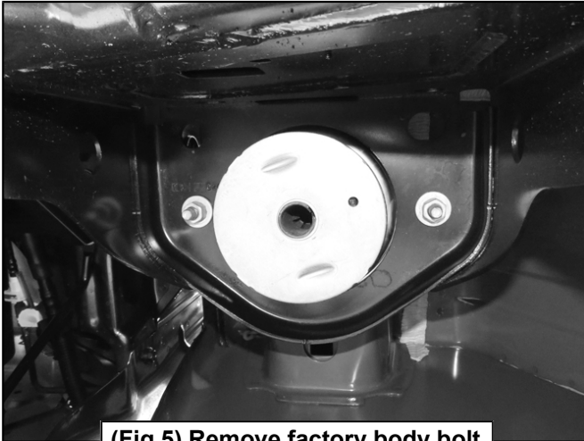
(Fig 5) Remove factory body bolt
