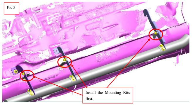
Step 4: Install the Mounting Kits first without fastening pieces, and then install the mounting brackets on the car. Next, install the side bar on the brackets and adjust the brackets.
