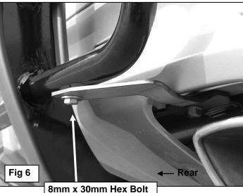
8mm x 30mm Hex Bolt 8mm Lock Washer 8mm Flat Washer
