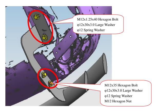
Step 3: Install the rear guard on the brackets and then adjust them to the proper positions. Step 4: Check if all hard ware are installed and then fasten all to complete the installation.
