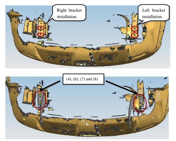
Step 4: After adjusting the rear guard to the proper place, please fasten all hardware and complete the installation.
