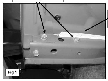
Trim or remove excess sealant as necessary to clear bracket for proper fitment
