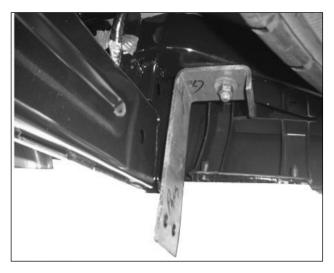
**4.** Fasten bumper bracket to cross member using (1) 1/2" locknut and (1) 1/2" flat washer. Tighten until slightly snug. Repeat for opposite side. **Passenger side shown**
