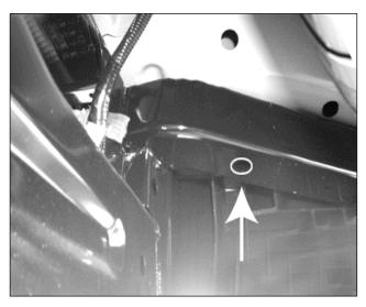
Locate (1) hole on each side of the square bumper crossmember. The holes are located between the two bumper brackets that are part of the formed frame rails. **Passenger side shown**
