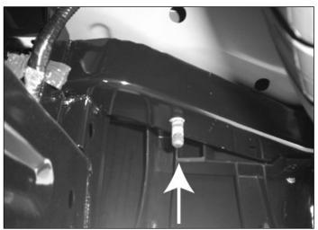
**3.** Insert (1) 1/2" bolt with rod extension through outside opening in square cross member and position so threaded end drops through hole in cross member. **Passenger side shown**
