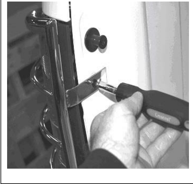
FIG. 3 Stock taillight mounting screws reinstall through inside brackets.
