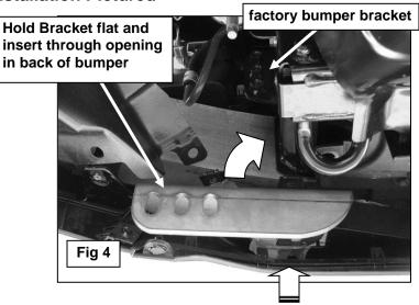
Line up Bracket and bolt to bumper bracket with (3) factory hex bolts
