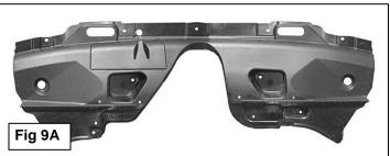
Install and align the Grille Guard as per instructions. Tighten all hardware before marking the area on the splash guard to cut for clearance
